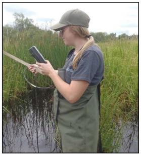
RVCA staff measuring water chemistry using a YSI multi-parameter water quality meter
