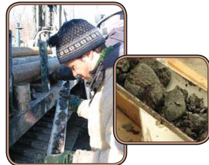
Drilling for core samples to determine the composition of the esker.
