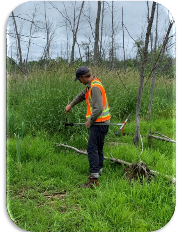
Soil sampling for wetland verification Long Sault East Industrial Park Township of South Stormont
